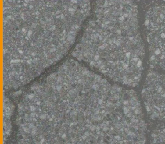
1 mm rastered true-orthophoto captured with 2 x 12 MP dual pavement camera
